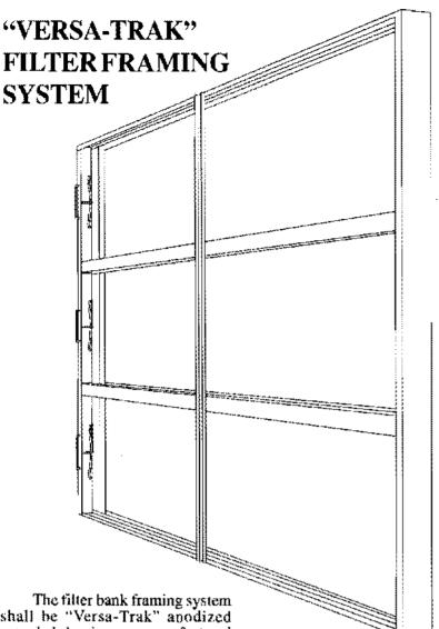
shall be "Versa-Trak" anodized extruded aluminum as manufactured by Applied Air Filters, San Jose, California.
