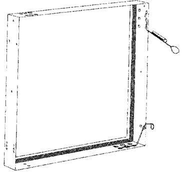
The Universal Type Holding Frame is made of 16 gauge galvanized steel, contains notches for various clips, has dimples for automatically centering the filters\*, and is fitted with a polyurethane foam gasket to assure a positive scal between filter and holding frame.
