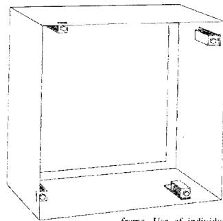
The Applied Air Filters HEPA Holding Frame shall be Model "HSL" as manufactured by Applied Air Filters, San Jose, California.
